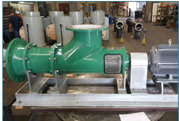
Circulation Pump at Hydraulics Laboratory
