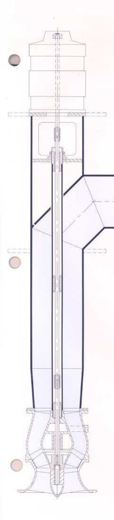
Driver: The pump is normally driven by a vertical electric motor or through a right angle gear drive coupled to a horizontal engine or electric motor. Hollow or solid shaft driver configurations with engineered shaft couplings and driver mounting design ensure proper installation and alignment in the field. Hydraulic and mechanical thrust created by the pump is carried by a thrust bearing in the driver.
